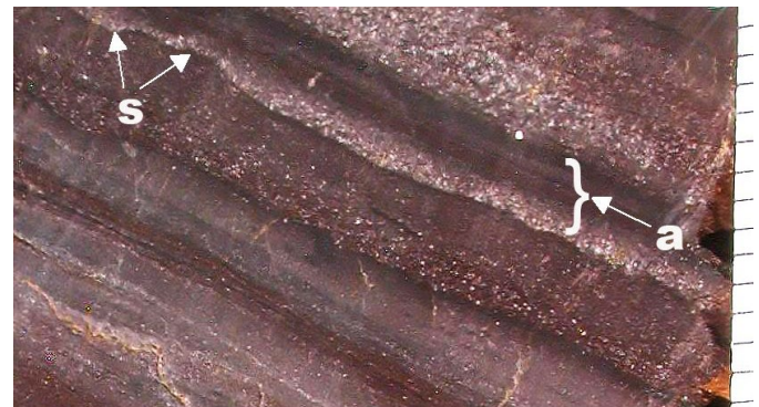
Fig. 6. Clastic sediment: a = normal graded bedding, s = sole and load marks. Hatch marks 1 mm.
